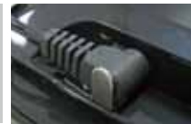
• DC Clamp (power Jack latch) to prevent power being unplugged
